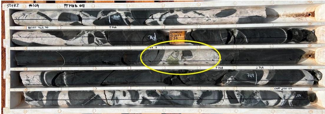
Figure 8: Hole 22PTMRD011 from 745.70 - 750.07m showing typical quartz – carbonate matrix supported jigsaw breccia that is dominant in the hole. Large slug of Chalcopyrite at 747.90m (yellow). Multi-element assays pending.
