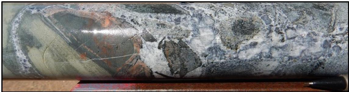
Figure 11: Hole 22PTMRD011 interval 773.7 – 773.9m showing a close up of the fluidised breccia. Note that some clasts have been reabsorbed into the matrix, while later incorporated clasts are sub-rounded. Minor sulphides are noted in the matrix. Wall rock exhibits sericite alteration with minor albite overprints.
