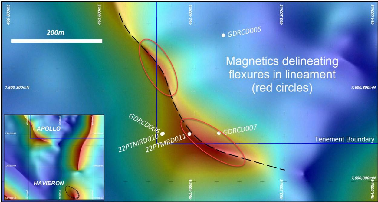
Figure 1: Reprocessed magnetics showing the ~1.5km long Apollo structure (highlighted in dashed line). Completed drillholes (white dots). Inset; Apollo location and anomaly size with respect to Havieron resource footprint (black outline).
