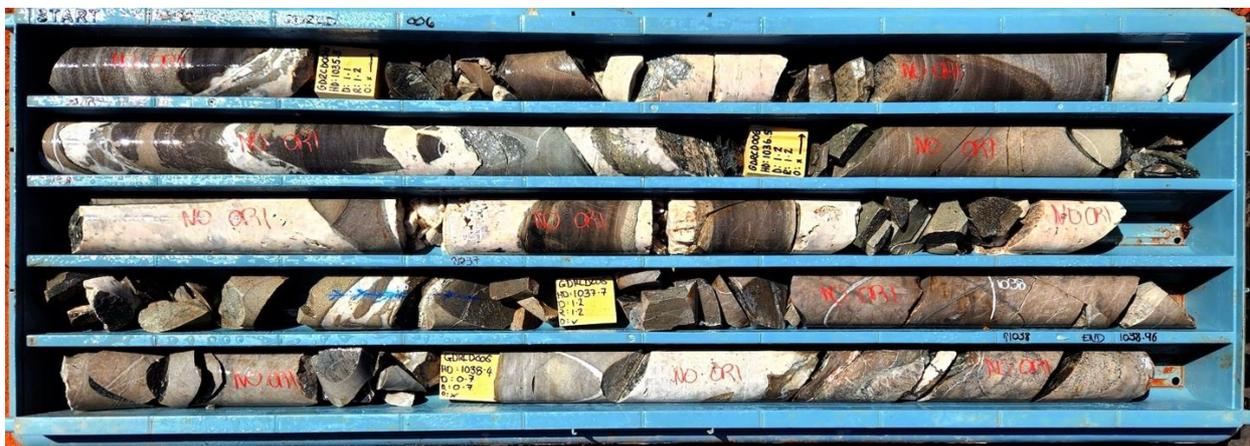
Figure 17: GRDCD006 tray at 1035.6m to 1038.9 shows vein and breccia formation with pyrite-chalcopyrite sulphide mineralisation associated with albite alteration of country rock.
