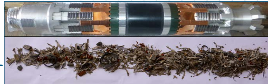
Copperhead drillable bridge and flow-through frac plug, after milling
