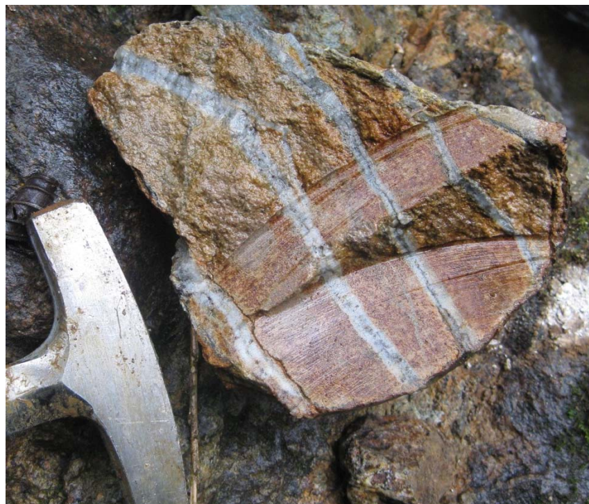
Figure 2: Photograph of quartz veins from the Alpala channel sampling area. The quartz veins contain centre lines of magnetite and copper minerals chalcopyrite, and some bornite.
