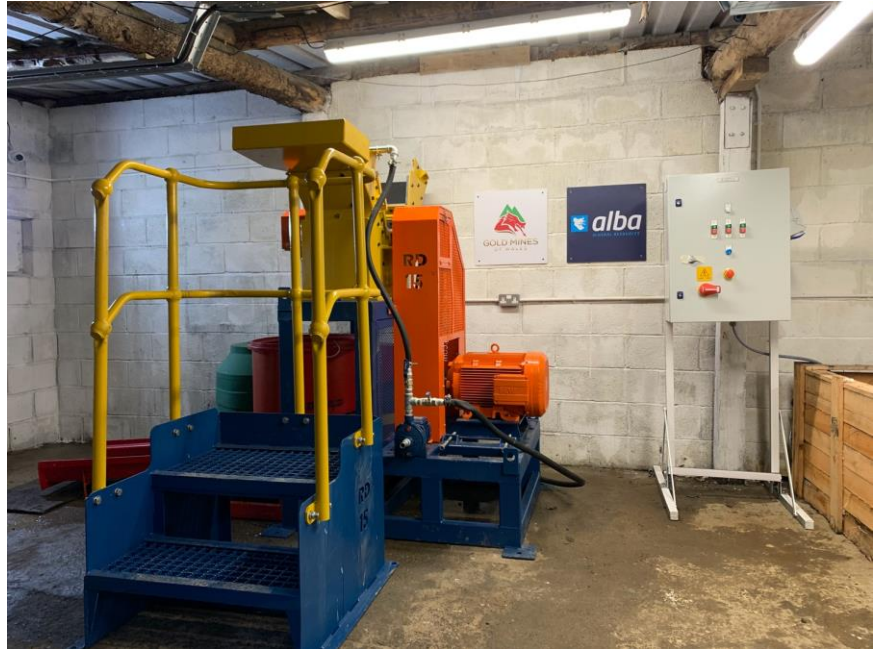
Figure 7: Installed impact crusher and gold concentrator, Clogau-St David's mine building.
