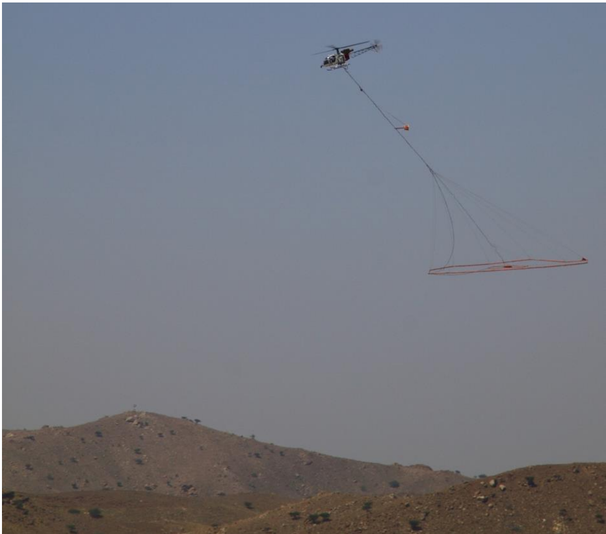
Figure 2. Geotech VTEM System conducting a VTEM survey in Oman
