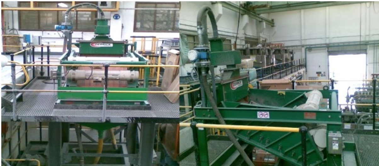
Figure 7 - Pilot scale Derrick Stack Sizer circuit used in beneficiation pilot program at Mintek.
