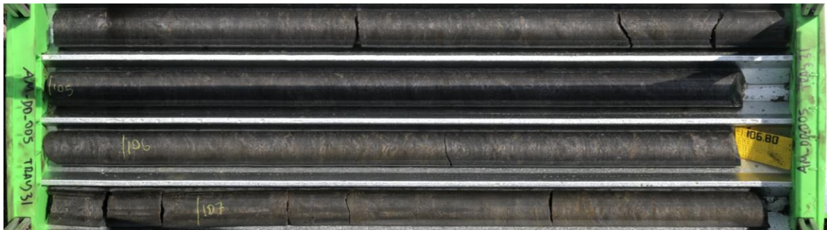
Figure 1: Photo of drill core intersection of LGL from hole DD 005 – 15.54m wide intersection
