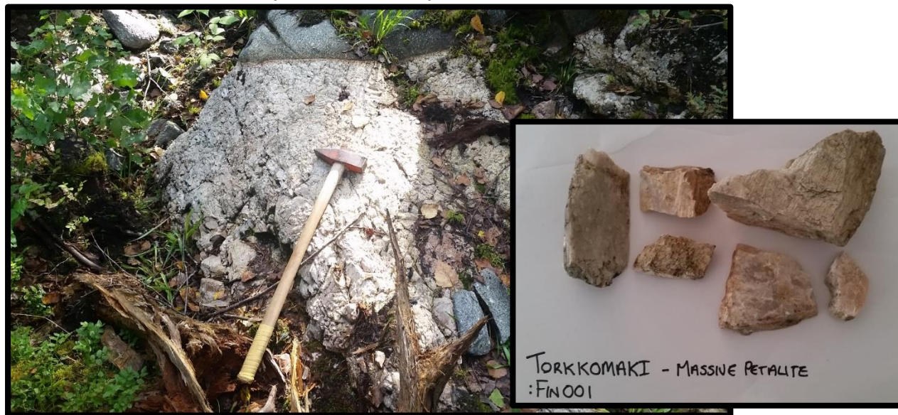
Figure 3. Pegmatite outcrop at the Torkkomaki Prospect showing massive occurrences of the lithium mineral Petalite (FIN001: 4% Li 2 O)
