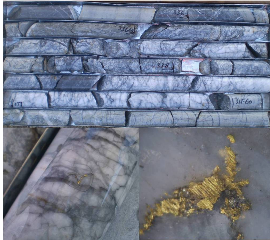
Figure 5 - Strongly mineralised Hapi Zone at HW contact D1351, 10250N and Visible Gold in the brecciated, sulphidic quartz vein 338 - 339m
