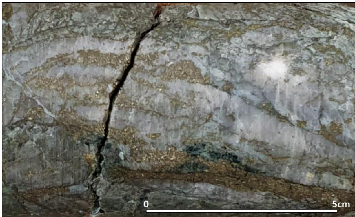
Figure 4: Selected drill core example of visible chalcopyrite-pyrite mineralisation, including trace visible bornite, at 68.8m depth in TAD-20-002.
