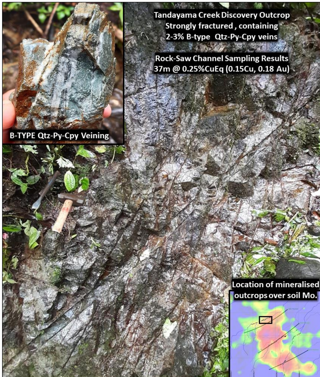
Figure 6: Rock-saw channel sampling over surface exposure in Tandayama Creek returned a significant assay result of 37m @ 0.25%CuEq (0.15Cu, 0.18 Au). This work was completed in mid-2016 as part of routine exploration on the tenement where B-type porphyry quartz veins hosting chalcopyrite mineralisation were discovered at surface.
