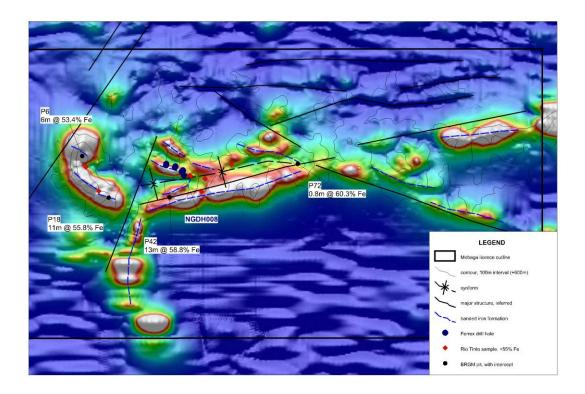
Core samples were submitted to Intertek's Johannesburg laboratory and assayed for a suite of elements specifically tailored for iron ore exploration by lithium borate fusion with an XRF finish. Industry-standard QA/QC programmes were employed by Ferrex and by Intertek.
