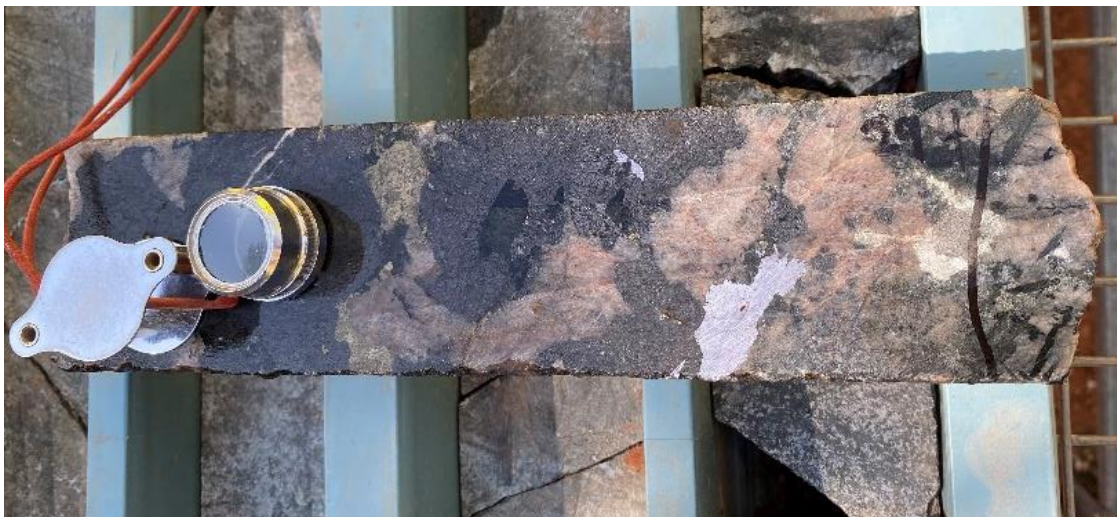
Photo 5: 21MHDD002: 293-294m (293.8m) - 1m @ 0.03% WO_3 , 0.04% Mo and 0.06% Cu – significant visible molybdenite and chalcopyrite visible throughout intercept, contrasting to assays
