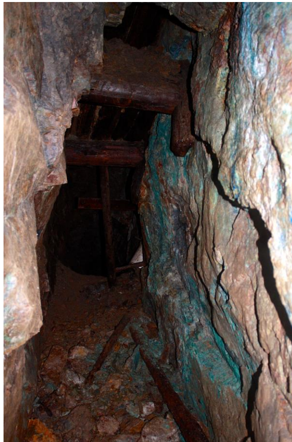
Image 1 – Underground workings showing visible copper mineralisation
