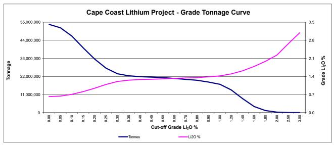
Figure 6: Grade tonnage curve for unconstrained pegmatite model
