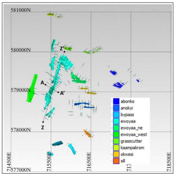
Figure 3: Plan View of Ewoyaa lithium resource wireframes and drilling with prospect names
