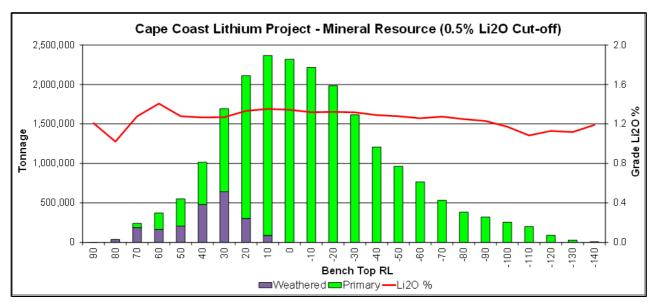
Figure 1: Ewoyaa Tonnage and Grade - 10m Bench Elevation
