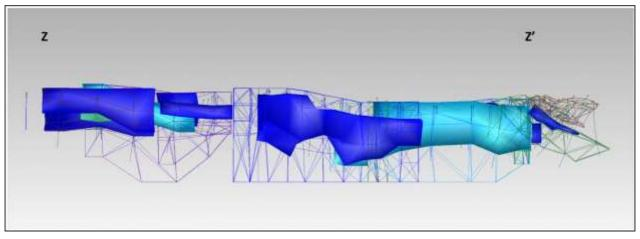
**Figure 4:** Long Section Z-Z' of Ewoyaa Main Wireframes and Drilling (View towards 300°; solid colours = resource wireframes, wireframe edges = pegmatite wireframes)
