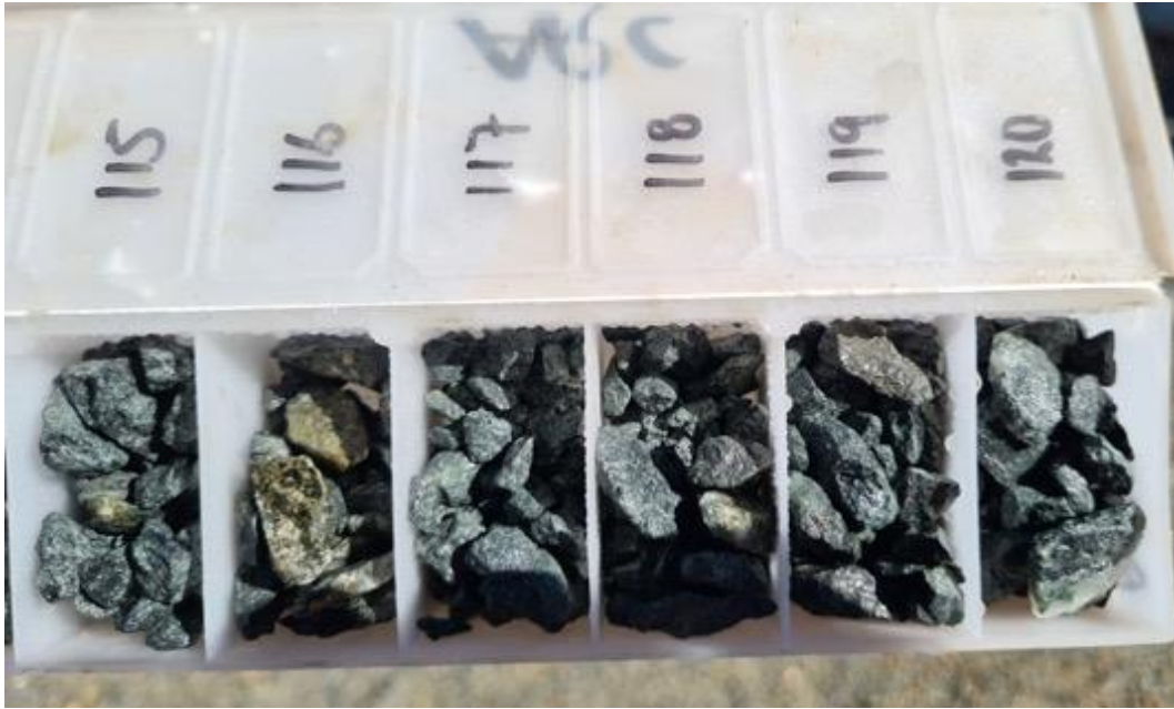
Figure 15: Sulphide occurrence in ARC403 comprising pyrite and pyrrhotite.
