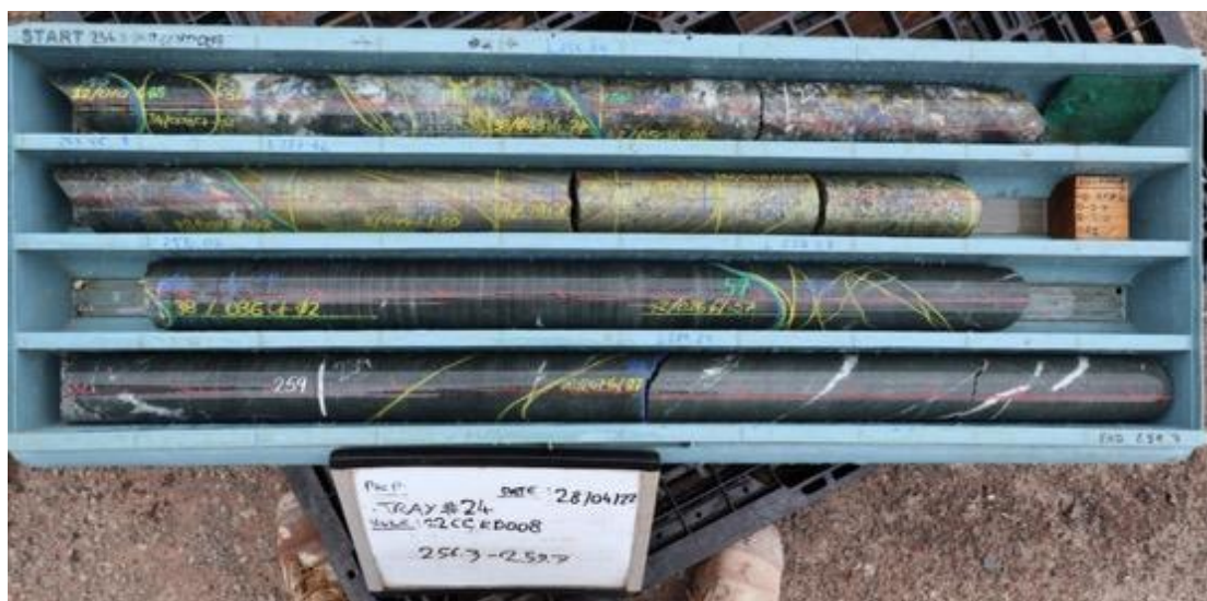
Figure 5: Part of the upper zone of the broader 16.6m showing the massive sulphide interval with brecciated upper contact which returned a result of 1.18m @ 15.65% Cu, 5.40g/t Au, 0.090% Co from 256.84m.
