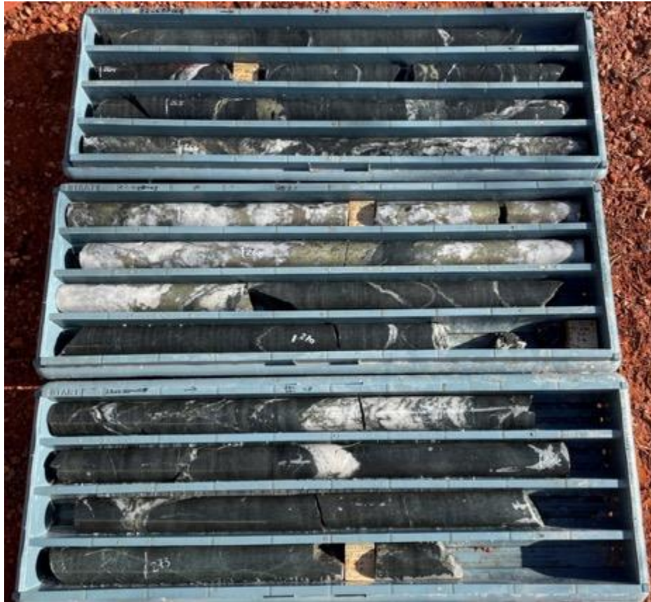
Figure 6: 22CCRD008 (263-273.5m) lower interval of significant vein hosted sulphide forming part of the broader 16.6m interval with a significant grade of 3.14m @ 6.38% Cu, 3.61% Cu, 0.059% Co from 265.92m
