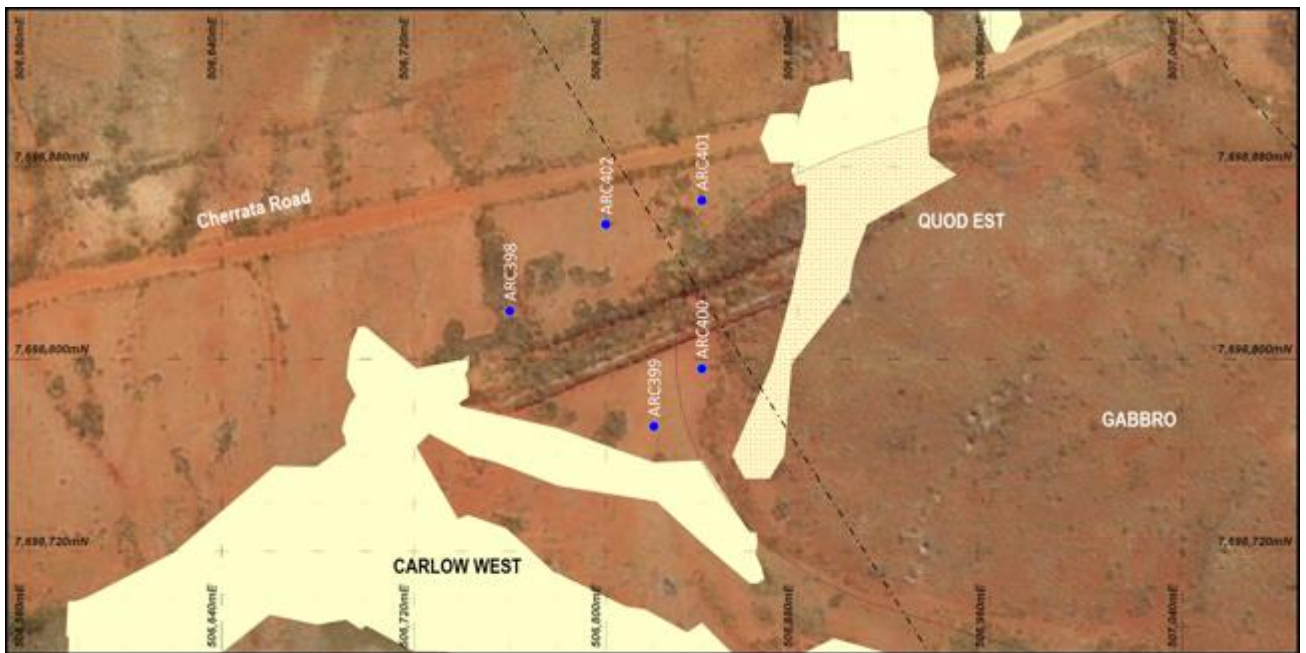
Figure 16: Location of Carlow West drill holes. Note trend of a NW structure in the vicinity of ARC401. Yellow solids are Carlow mineralised polygons.
