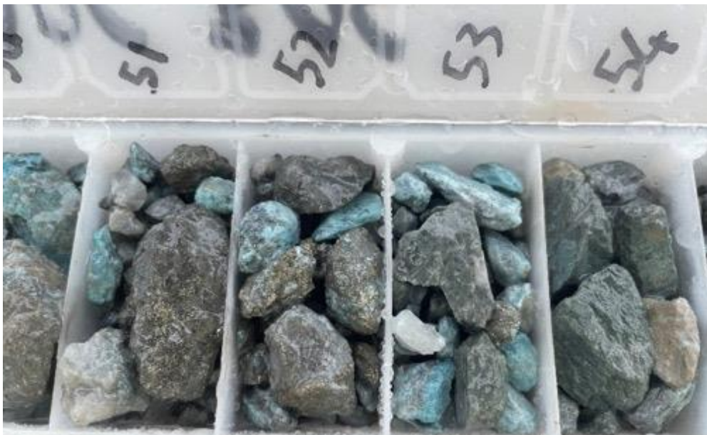
Figure 10: Interval of sulphide and fuchsite in Hole ARC395. Assay results are pending for hole.
