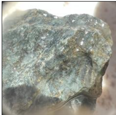
Figure 12: ARC396 [107-108m] 1% pyrite and pyrrhotite in silicified sericite matrix. Assay results are still pending for this hole.
