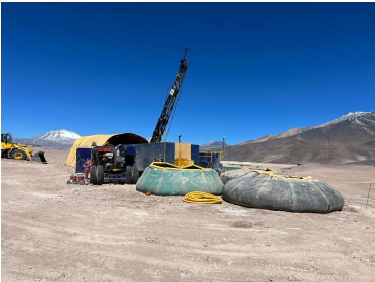
LV03 slant drilling rig – Laguna Verde
