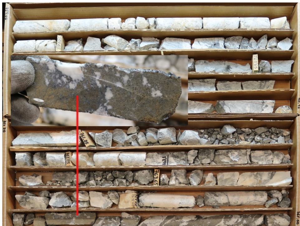
Figure 2: photograph of Peñarroya's historic hole, SJ22 (twin target of TOD-023), from 759 to 765m downhole, at the IGME National Litoteca core library, Andalucia, during the Company's 2018 re-logging programme. The BQ dimension core shows strong Zn and Pb mineralisation, especially around 764.50m.
