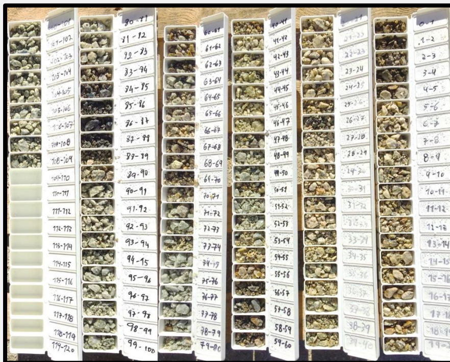
Figure 3. RC drill chips from 17GRARC17 which returned a result of 109m at 1.04% Li 2 O (uncut) from surface
