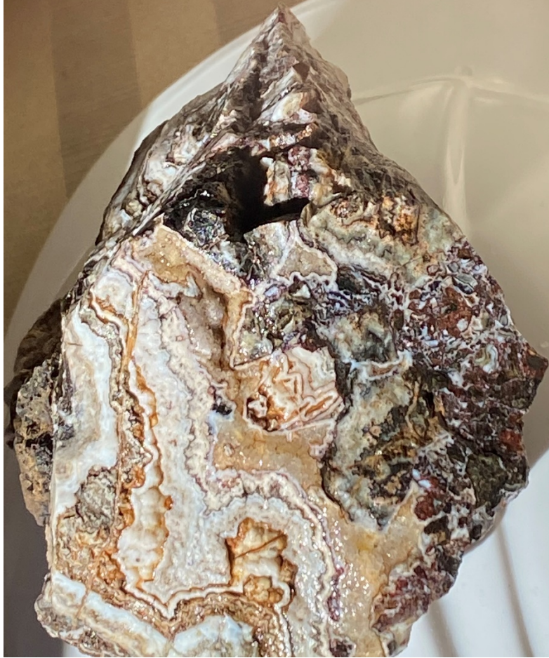
Figure 3: Close up of surface sample of epithermal alteration associated with main historic silver mineralisation at San Celso, March 2022
