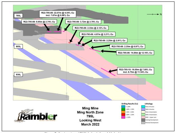
Figure 7: Section view of 795L holes 6, 8, and 10, looking west
