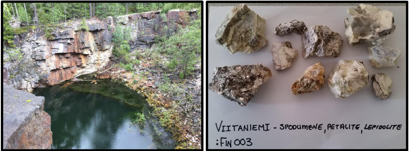
Figure 5. Old pit on the Vitaniemi pegmatite and abundant lithium minerals located in the pegmatite, predominantly Petalite, Spodumene and Lepidolite (FIN003: 1.29% Li 2 O)
