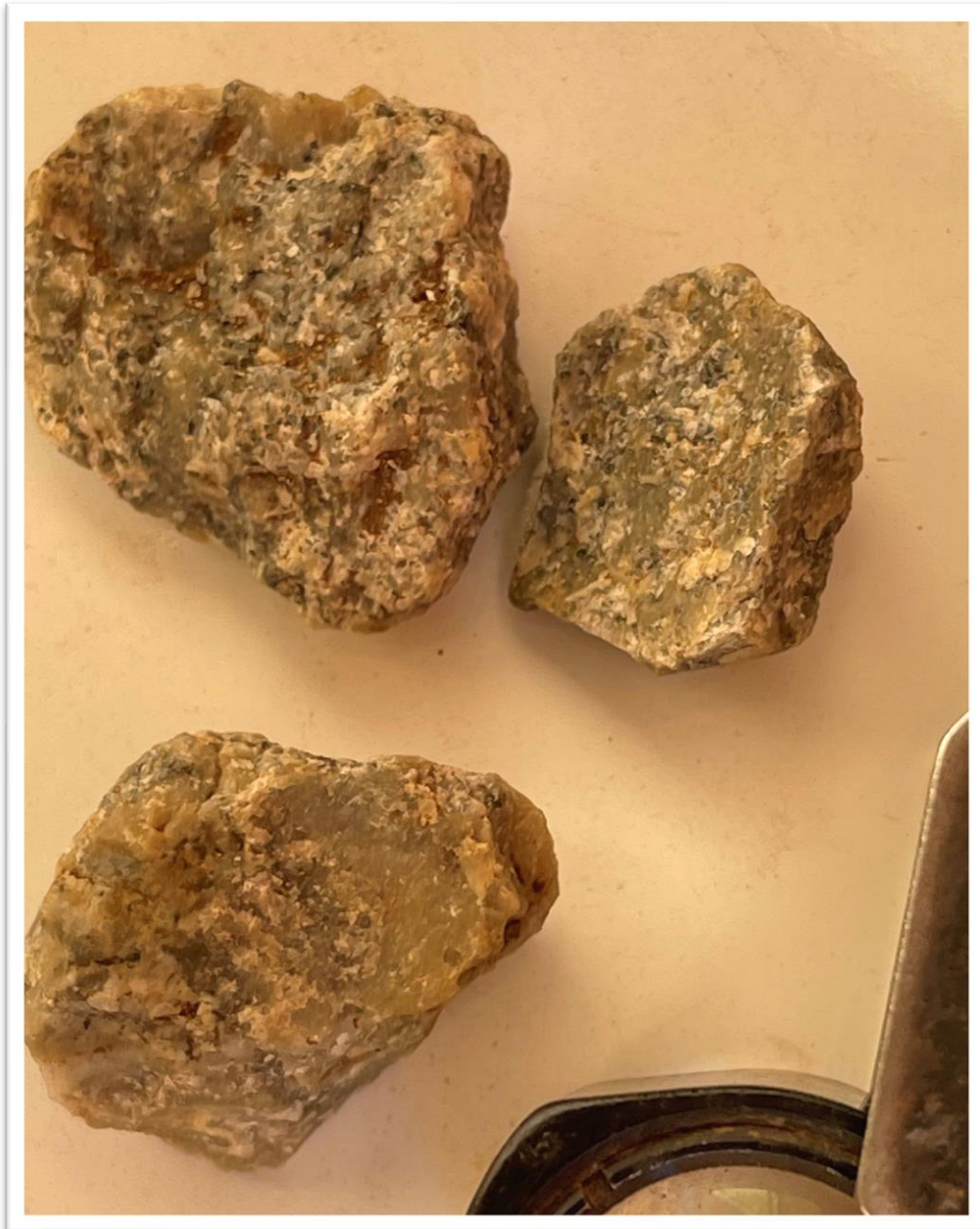
Figure 3: Silver bearing granite chips from RC hole AMEHRC002 at 64m depth, Elizabeth Hill, October 2021 (pXRF reading 120 g/t silver).
