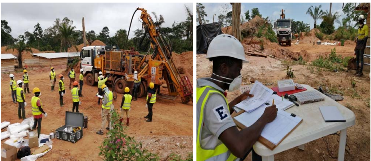
Figure 1: Aircore drilling now underway at Zaranou; pre-start toolbox meeting (left) and logging (right).
