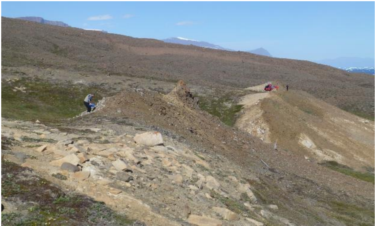
Figure 4 - Illukunnguaq area on Disko showing Gossan. 1.9% Cu, 3.3% Ni, and 1.1% Cu, 2.8% Ni in outcrops.
