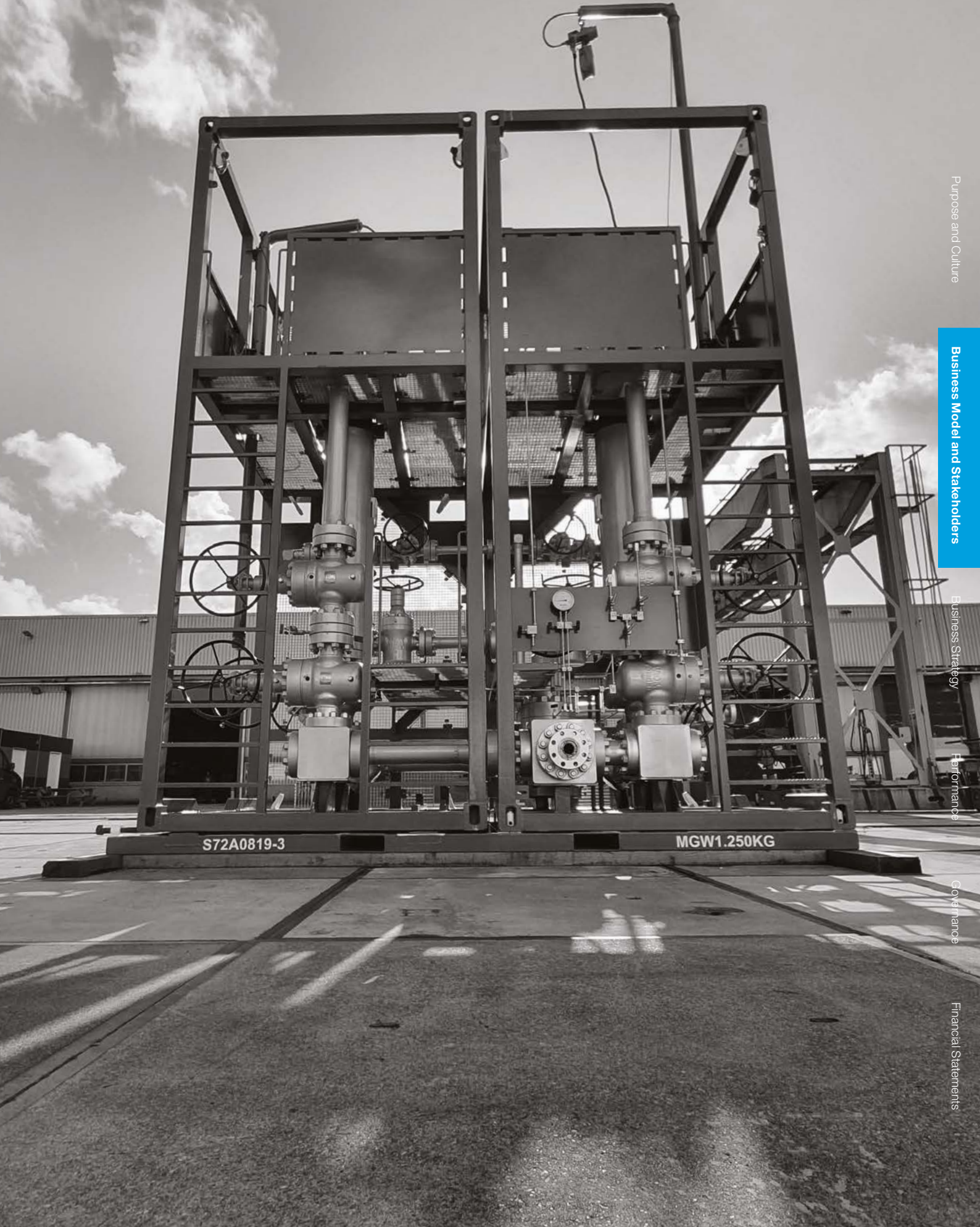
A Dual Pot Sand Filter manufactured by the Well Testing business in the Netherlands.
