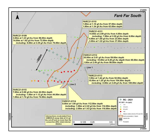
Cross sections for drill fence lines L1 and L2 at Faré Far South, highlighting best intersections from 2021 Phase 1 reverse circulation drilling programme
