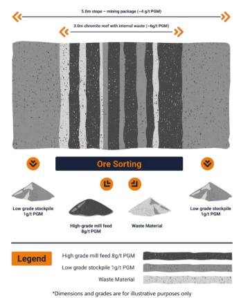
Figure Nine | Ore Sorting Schema
