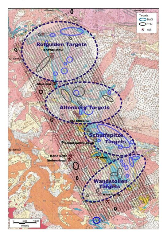
Figure 1 - EM / magnetic targets derived from the recent survey, over the Rotgülden licence area, flight lines are in black overlain on the geology of the area.
