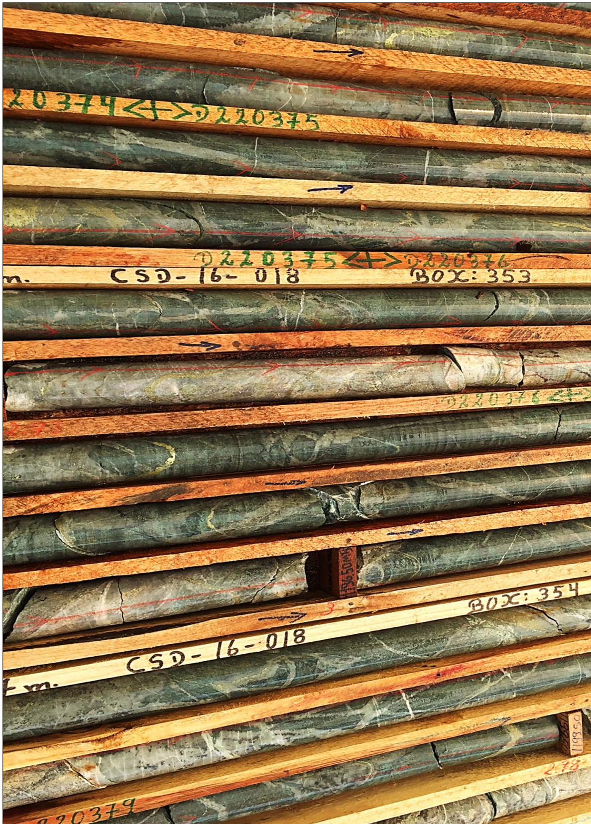
Figure 5: Examples of mineralisation encountered in Hole 18 at around 1200m depth.
