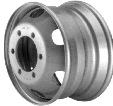
Auto: Commercial Vehicle rim (4.5mm & 6.2 mm thickness)
