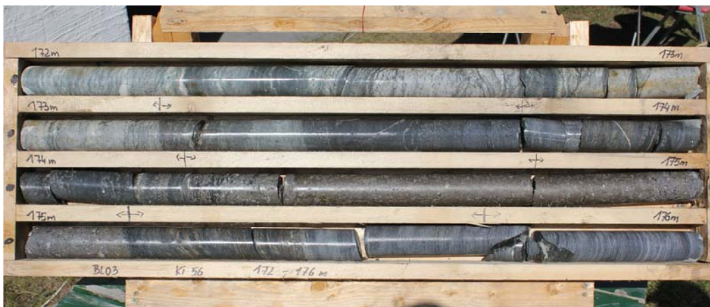
Image 1 – Core from diamond drilling of hole BL03 at Rotgülden showing intercepts of massive sulphides
