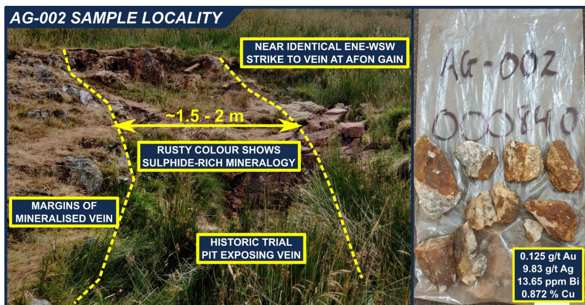
Figure 4: Photograph of the AG-002 Sample locality at Afon Gain, highlighting the thickness of the vein observed in outcrop, with sample assays in the bottom right corner.
