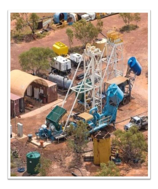
Figure 2: Headframes, gensets, compressor, workshop on site in NT prior to dismantling for transport to Elizabeth Hill
