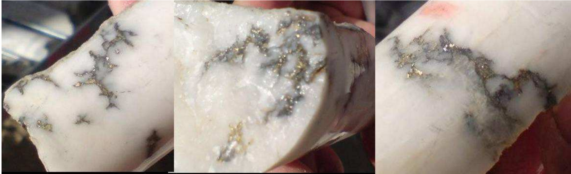
Figure 8 – D1280 558 – 559m; massive milky quartz vein, gold and galena veinlets, a zone beneath Hapi Zone
