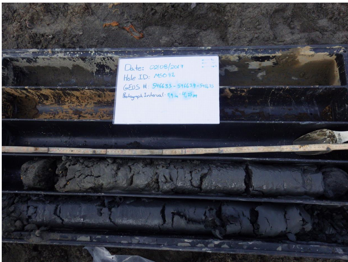
Figure 4. Typical sonic drill core. A high grade "ilmenite blanket" that drapes the bedrock unit identified over license area
