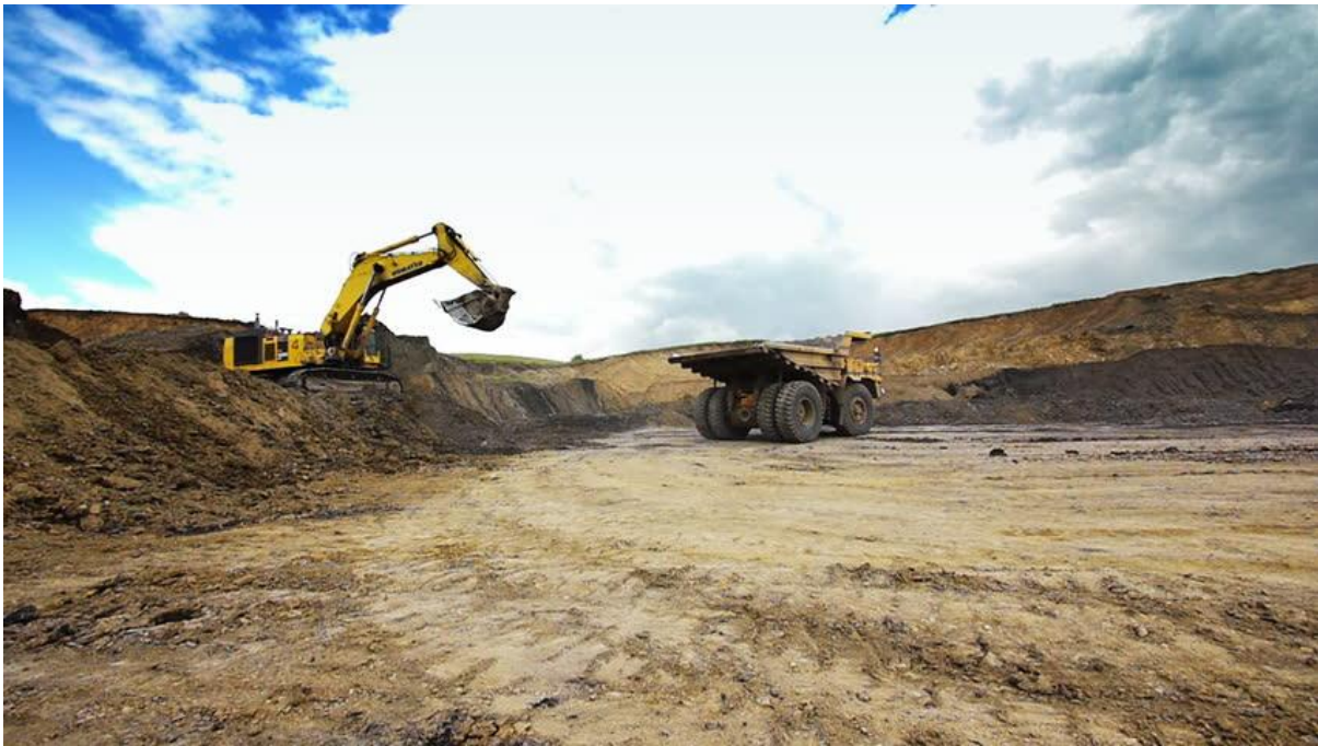
Figure 1: Example of a conventional truck and shovel open pit operation.
