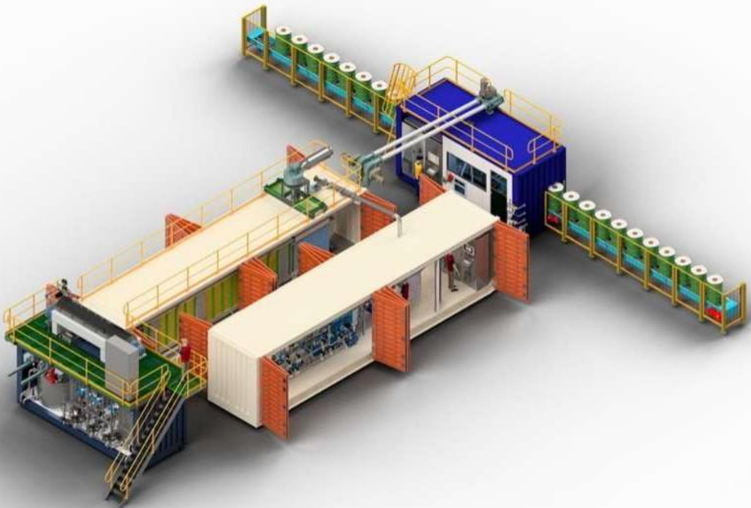
Figure 5.6: Isometric plan of UOC drying and drum packaging plant
