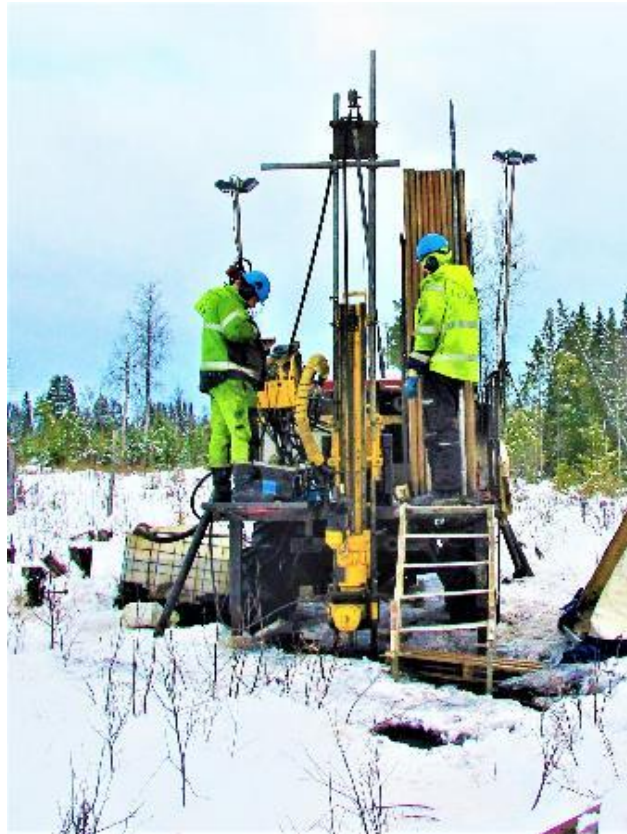
Plate 1: Diamond drilling in -20°C temperature – Häggån winter drilling
