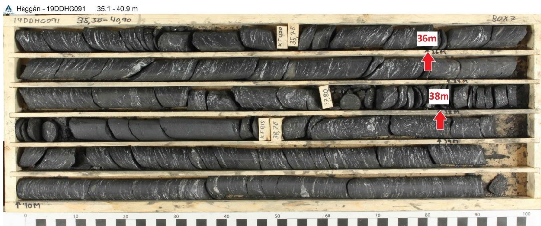
Figure 4: Häggån mineralisation. The top 3 rows of core (to 38 metres) average 0.61% V 2 O 5
